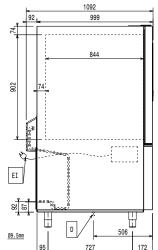
Drain Electrical inlet (power) FΙ Refrigerant Outlet
